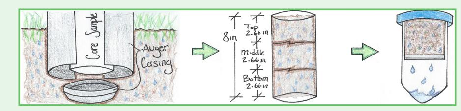
Figure 5: Retrieval of Pore-water from Soil
