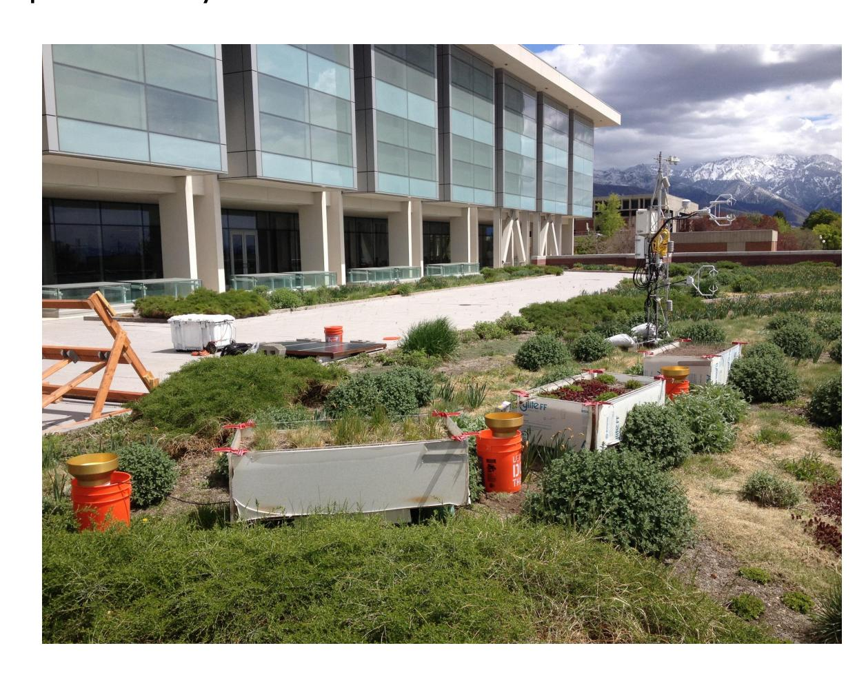
Figure 3. Three lysimeters used on Marriott Library green roof. From left to right: bluegrass, sedums, non-vegetated.
