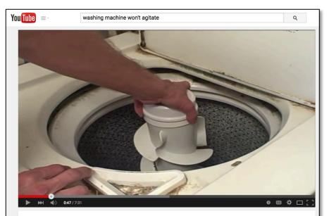
How to fix an Agitator on a Washing Machine
